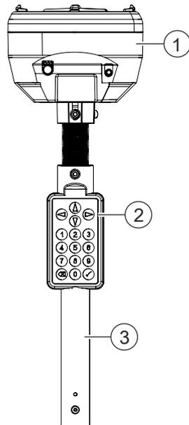
*Service device with test head, keypad and handle*
