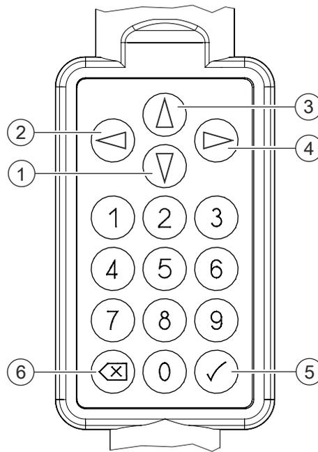
Keypad with numerical keys and navigation keys
